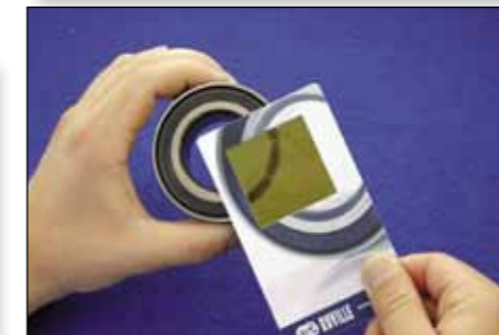
Using the detector card on a sensor bearing, with detection of the pulse generator in the lower picture.
