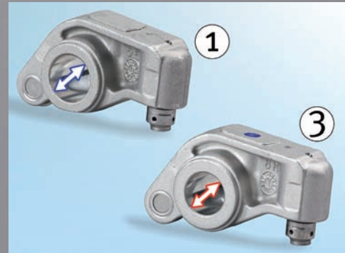
Figure 2: The diameter of the rocker arm is greater on the intake side (1)
